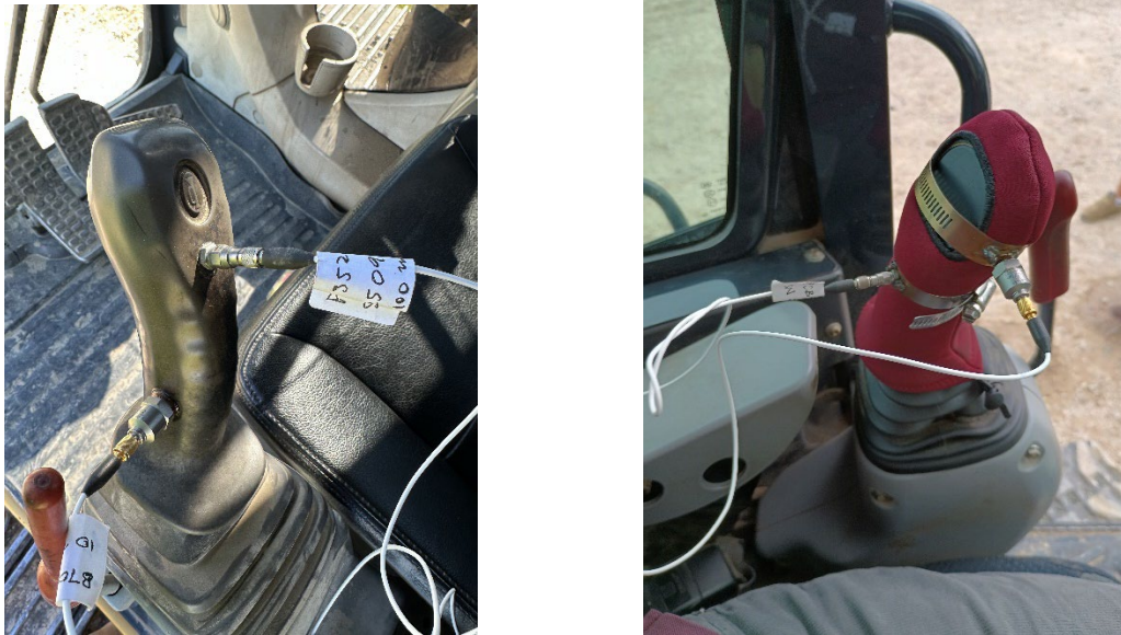
Figure 3. Excavator testing setup
